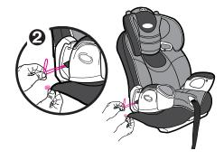
3. Pull the seat pad out of the way to reveal red buttons as shown in **3**. Slide the buttons to release the back support from the base and lower it into a flat position.
